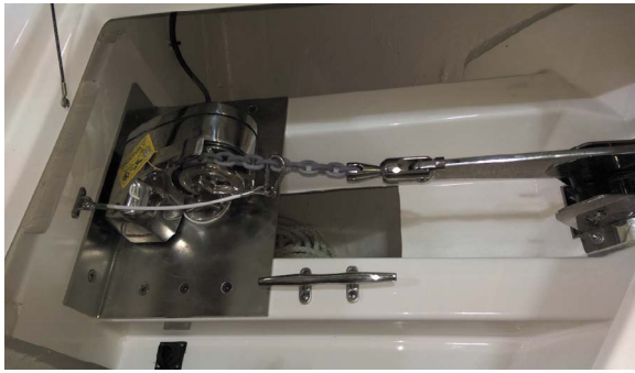
Anchor Line Secured Using Cable
