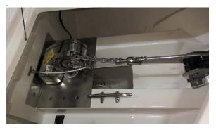
Anchor Line Secured Using Cable
