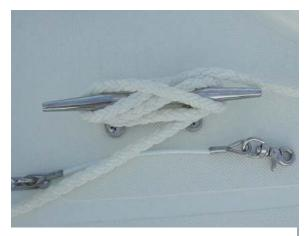
**Anchor Line Secured to Cleat**
