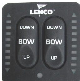
Trim Tab Switches
