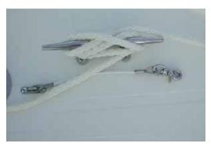
**Anchor Line Secured to Cleat**
