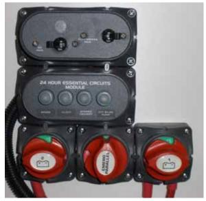
**Battery Switches and Main Breakers**
