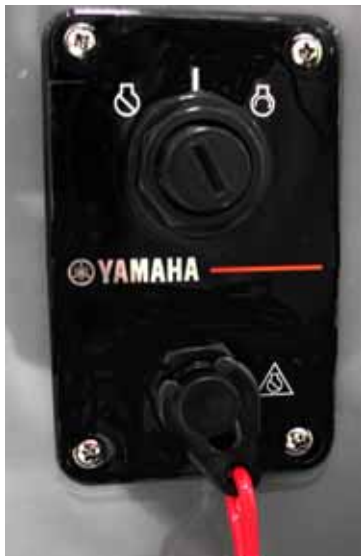
Engine Stop Switch
